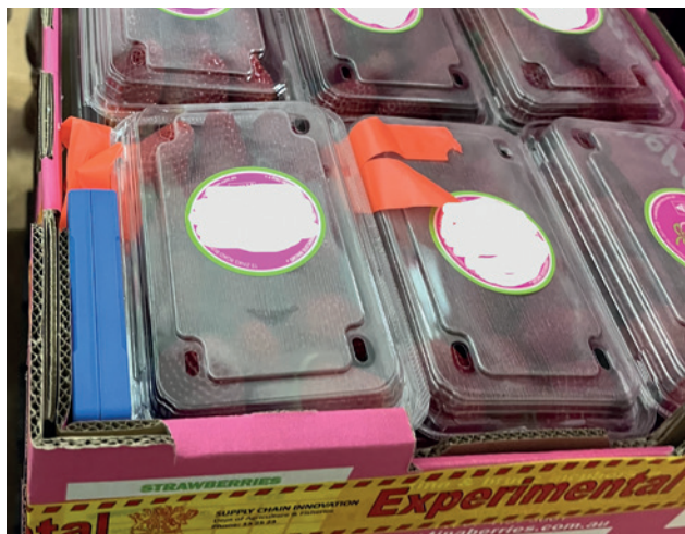
Figure 1. Strawberry tray with logger inserted to monitor supply chain conditions
