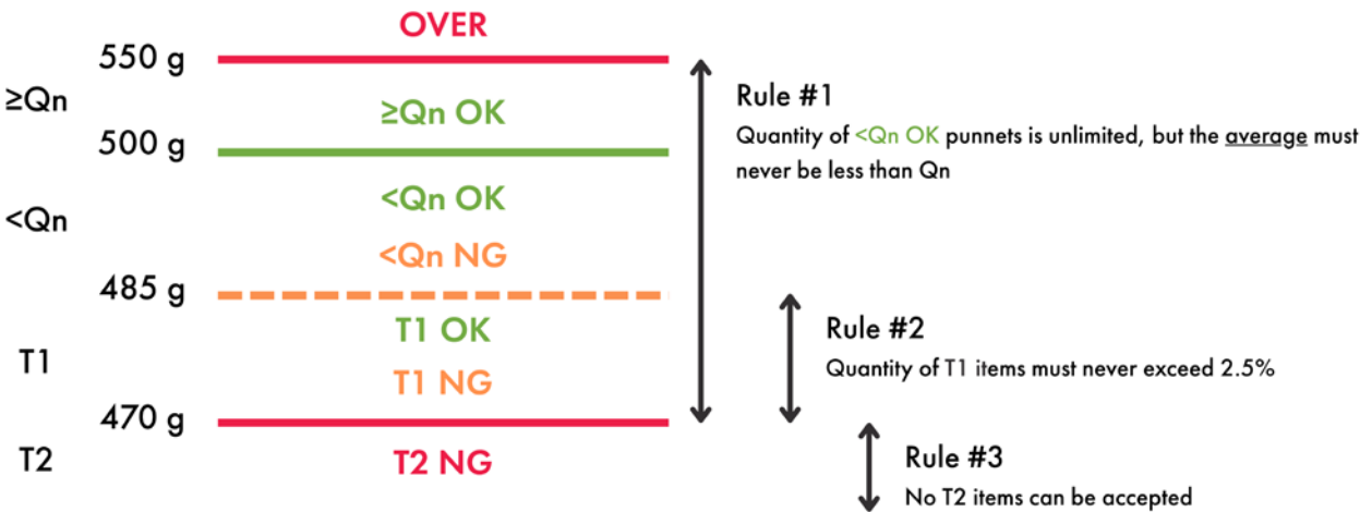
Figure 2. Simplified summary of the AQS (e-weight) method showing how the three measurement rules are applied for a 500g punnet. Rejected punnets <Qn NG and T1 NG may be added to a batch later in the packing process when the statistics support them (when the average weight is higher than the nominal weight and the quantity of T1 items is below 2.5%) or be re-worked.
