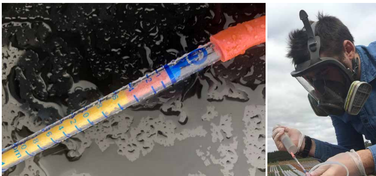
Figure 3. Colorimetric tubes contain reagents that change colour proportional to the amount of fumigant in the soil. (L) tubes for the fumigant 1,3-dichloropropene change from yellow to pink and (R) measuring fumigant residues in soil before planting using colorimetric tubes. Photo credit VSICA Research
