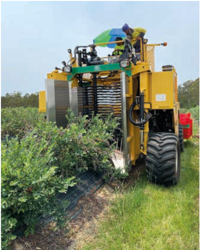
Jas Benning standing on top of the harvester ensuring proper positioning, speed and vibration is used
