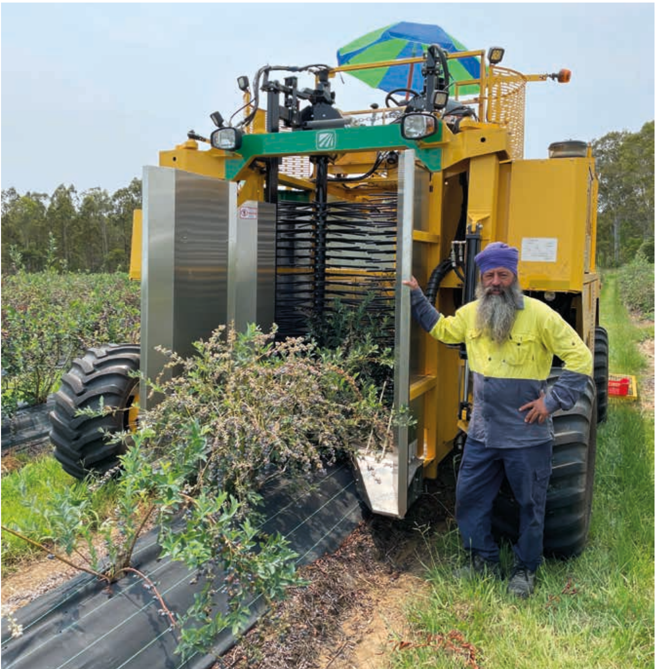
Jas Benning standing next to the blueberry mechanical harvester in a rabbiteye block. Photo credit: NSW DPI
