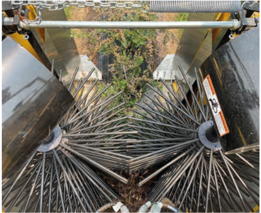
Rotating and vibrating rods used to detach ripe berries. The speed and vibration of the rods dictates the strength at which the blueberry bush is shaken
