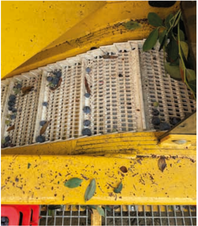
Fruit that has been knocked off the bush is moved into red trays on the white conveyor belt, while rubbish is blown off from a chute above it
