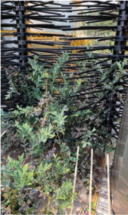
Rotating and vibrating rods used to detach ripe berries. The speed and vibration of the rods dictates the strength at which the blueberry bush is shaken
