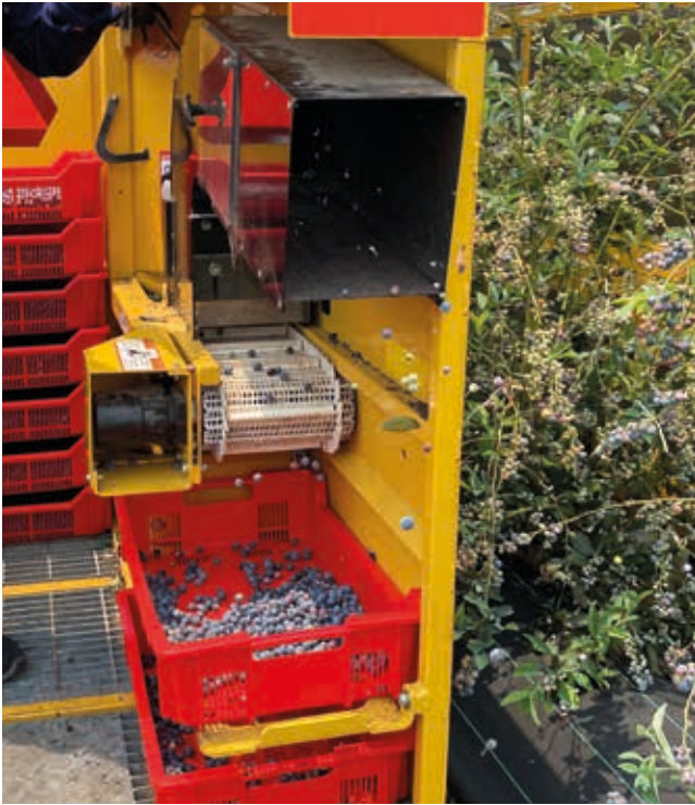
Fruit that has been knocked off the bush is moved into red trays on the white conveyor belt, while rubbish is blown off from a chute above it
