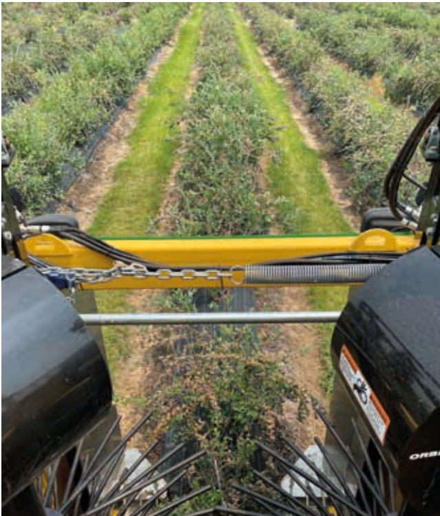
Positioning the mechanical harvester in the middle of the row ensures no fruiting laterals are missed. One of the difficulties faced harvesting a young bush is the proximity of the fruiting lateral to the weed mat
