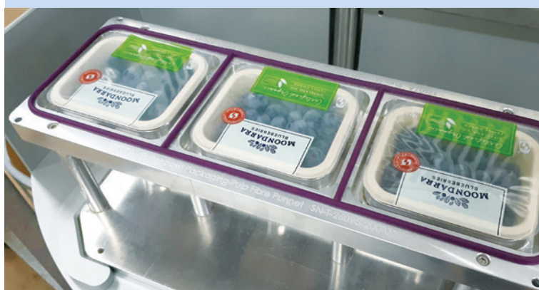
Punnets being capped on the Proseal Australia GTR heat seal machine – semi-automatic with rotary table. Capable of capping 45 punnets per minute. Photo credit: Moondarra Berries.
