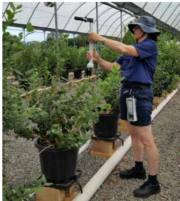
DPI Technical Assistant, Leanne Davis measuring canopy area of Blueberry plants using a leaf area index meter.
