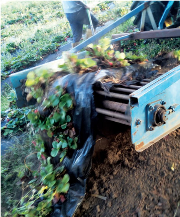
Modified garlic digger lifting plastic and plants, including the crowns. Photo credit: Portland Strawberries
