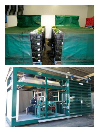
Figure 1. Forced air (top) and vacuum cooling systems (bottom). Photo credit: AHR, Quik-Cool
