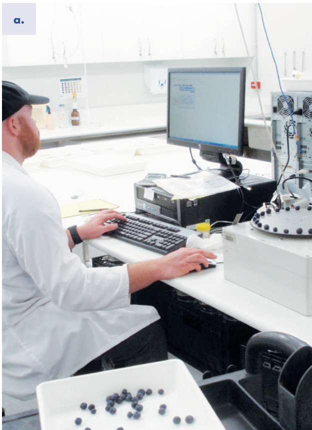
Figure 3a and b. Objective measurement of compression firmness of blueberry fruit using a FirmTech firmness tester at NSW Department of Primary Industries. Photo credit: John Golding.
