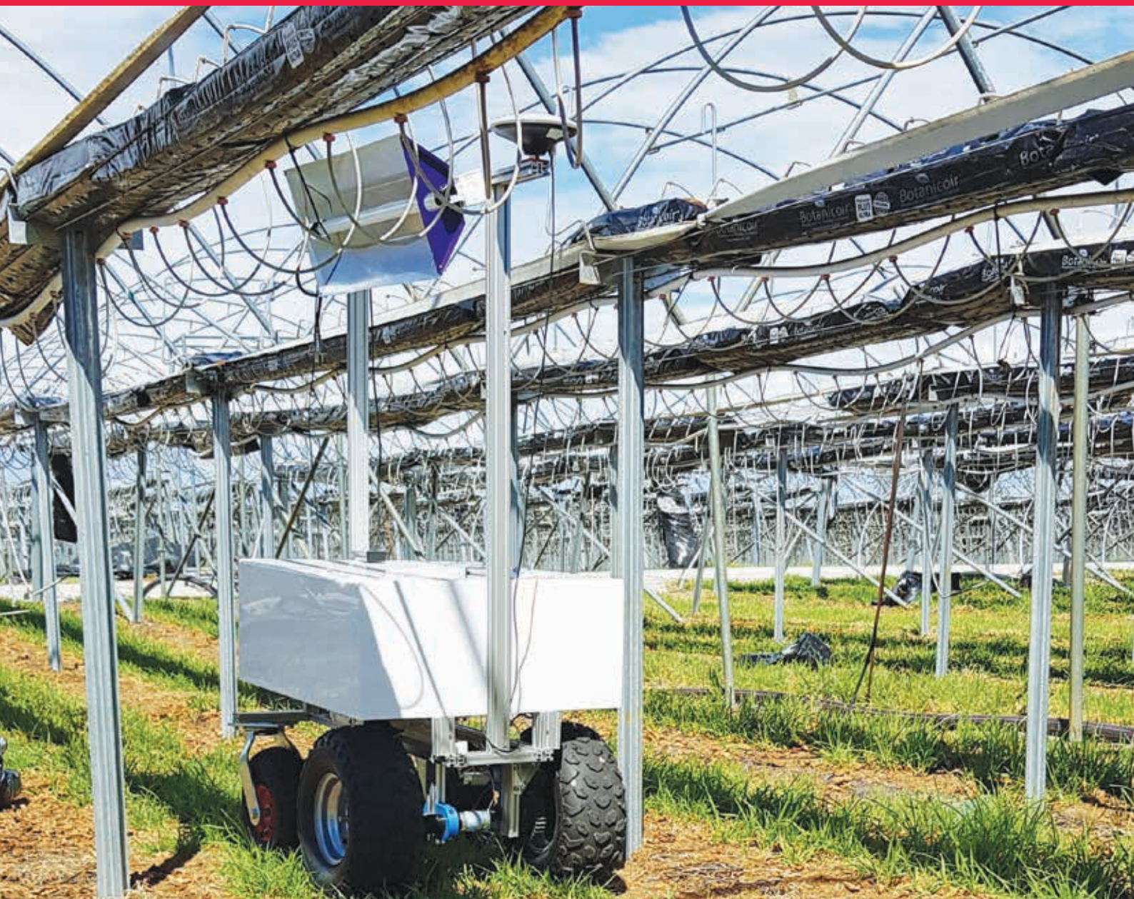
Figure 2. Testing of the Outback Robotics prototype is currently underway in Western Australia. The prototype is the size of a person and can move up and down rows of tabletop strawberries with ease. The system is adaptable to different tabletop configurations. Photo credit: Robert Walker, Outback Robotics
