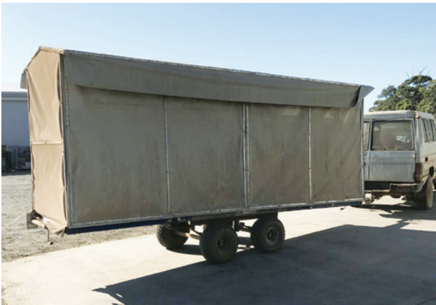
Figure 3. This covered wagon protects harvested fruit from the sun, wind, and rain as it is transported from the field to the shed. Photo credit: Anthony Yewers
