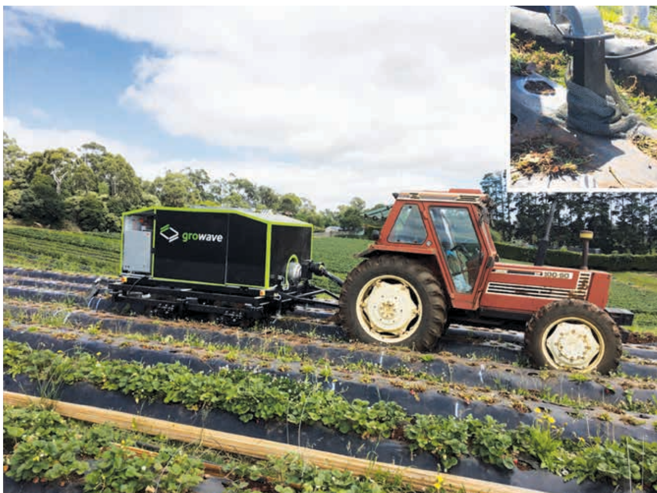
Figure 2. Prototype 5 kW microwave unit used for crop termination. Inset: Antenna targeting microwave energy to old strawberry plants. The unit is designed by the company GroWave Pty Ltd ( www.growwave.ag ). Photo credit: VSICA Research
