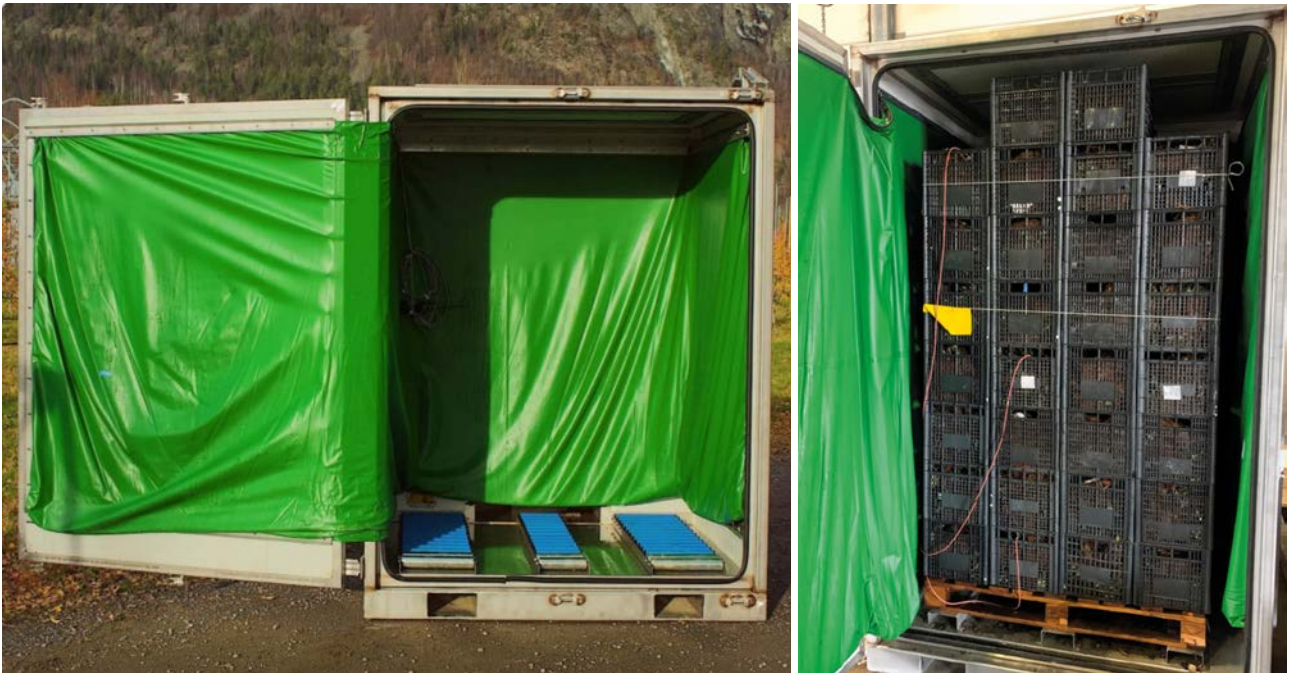
Figure 1. The chambers used for aerated steam treatments in Norway and Florida were constructed by Plantsauna AS (now Moleda AS) https://moleda.nl . Photo credit: Moleda
