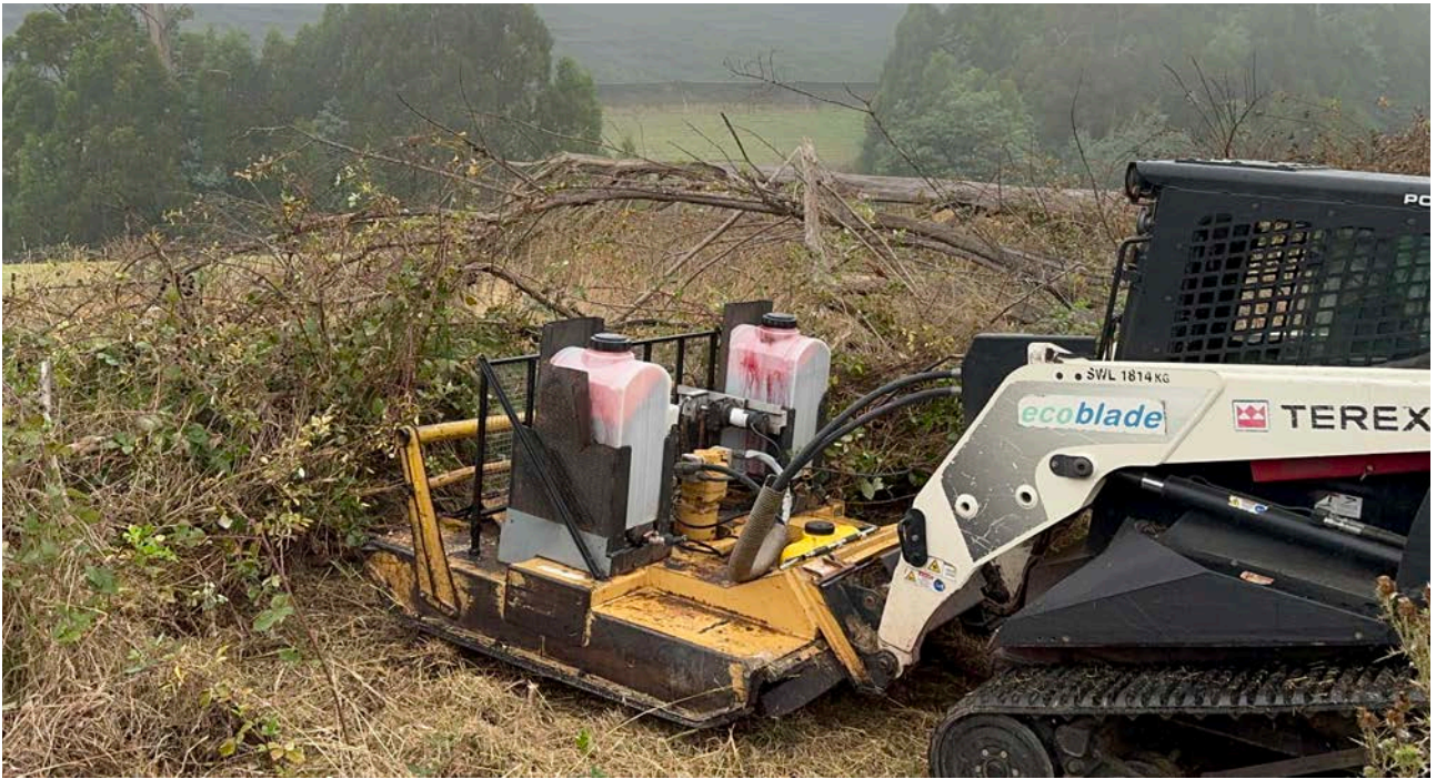
Figure 6. Ecoblade, “cutting and painting” a problematic blackberry area, in preparation for either a return to pasture or a revegetation program. Photo credit: Bronwyn Koll
