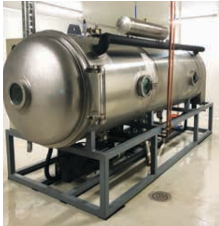
Freeze drying equipment
