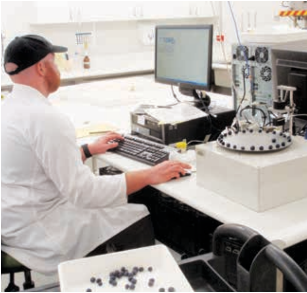
Figure 2. Measuring blueberry firmness with FirmTech instrument at NSW DPI
