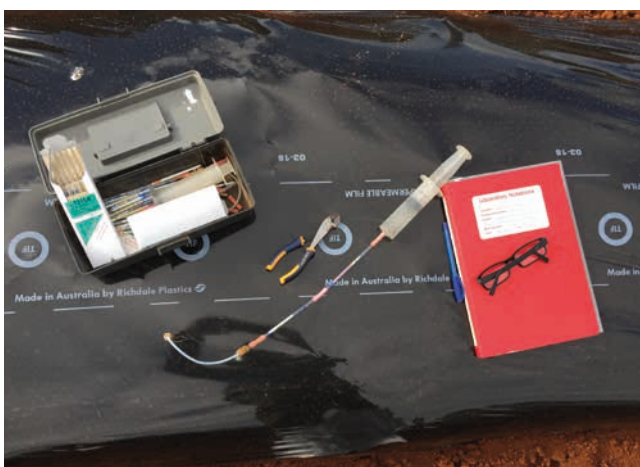
Figure 3. Dr Dylan McFarlane drawing gases through colorimetric detector tubes (Gastec®) to determine the concentration of fumigants in soil. Photo credit: VSICA
