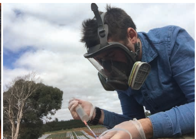
Figure 3. Dr Dylan McFarlane drawing gases through colorimetric detector tubes (Gastec®) to determine the concentration of fumigants in soil. Photo credit: VSICA
