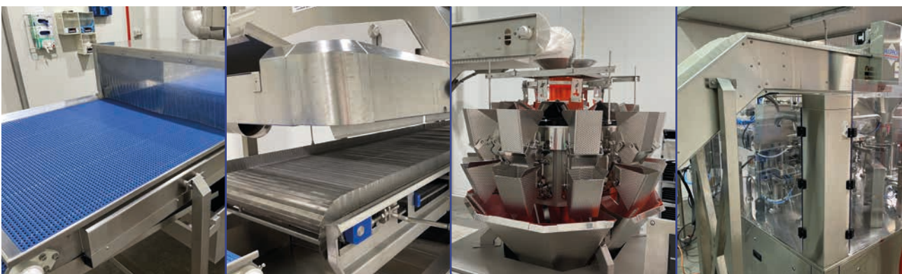
Snap freezing capability developed by the Oz Group in recent years. Berries are washed, snap frozen then portioned and packed.
