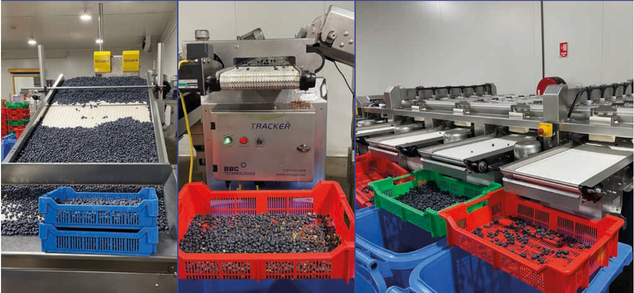
Mechanised sorting equipment in use at the Oz Group Co-op packhouse takes fruit from the orchards (above) and separates the defective fruit from the premium berries. Photo credit: Gaius Leong
