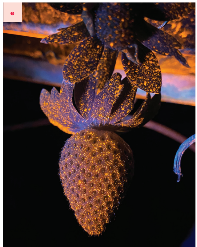
Figure 1 (b, c, d, e) The Silvan Turbomiser™ airboom sprayer achieved excellent coverage of upper and lower leaf surfaces and fruit and had uniform droplet size. Photo credit: (b, c) Malcolm Jones, Syngenta (d, e) Helen Newman, APC
