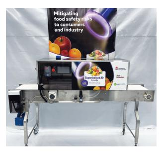
Figure 1. The cold plasma prototype incorporates multiple treatment options and is fully automated, allowing safe application of the technology in packing operations. Photo credit: Dr SP Singh, NSW DPI
