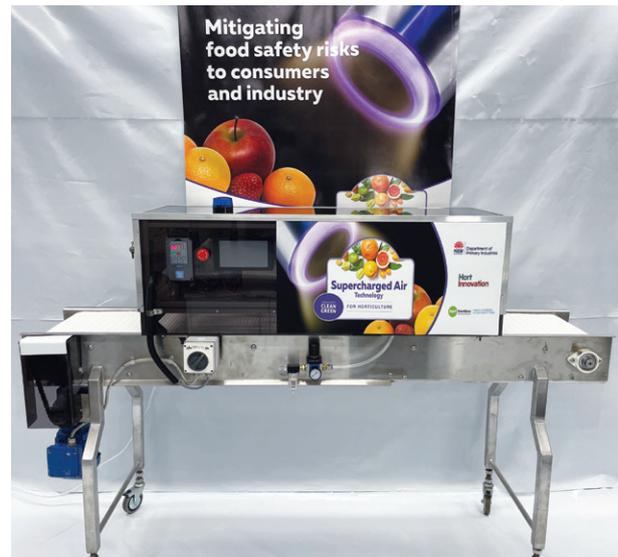
**Figure 1. The cold plasma prototype incorporates multiple treatment options and is fully automated, allowing safe application of the technology in packing operations.**
