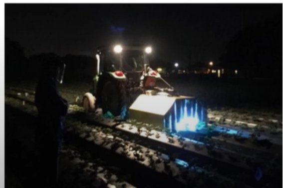
Figure 2. Prototype UVC applicator designed to suit the dimensions of strawberry beds in Florida.
