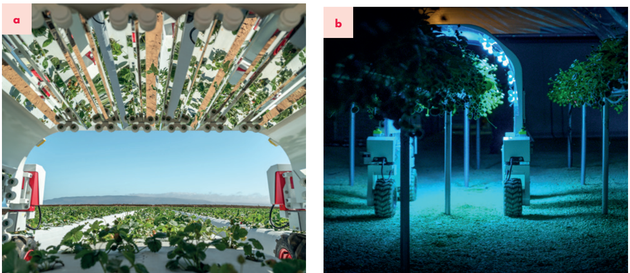
Figure 7. Saga Robotics 'Thorvald' autonomous robot that can apply UVC without the need for a tractor.
