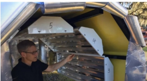
Figure 2. Prototype UVC applicator designed to suit the dimensions of strawberry beds in Florida.
