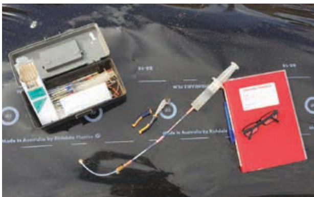
Figure 3. Measuring fumigant gas concentration under totally impermeable film (TIF)
