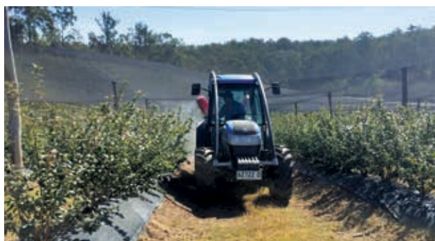
Figure 1. Croplands Quantum mister sprayer in blueberries. Note the angle of the setup to allow optimum coverage. Photo Credit: Melinda Simpson
