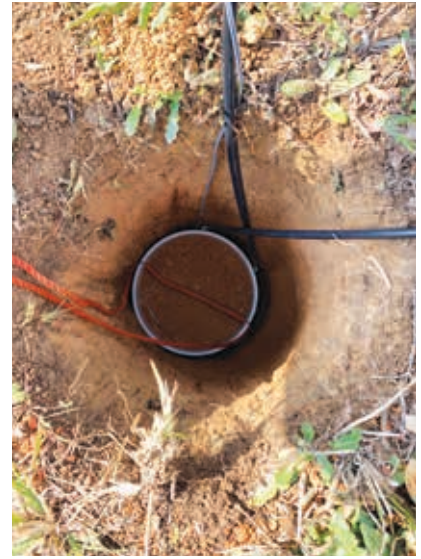
Figure 4. Installing nutrition and irrigation monitoring equipment at one of the demonstration farms. Photo Credit: David Mitchell NSW DPI
