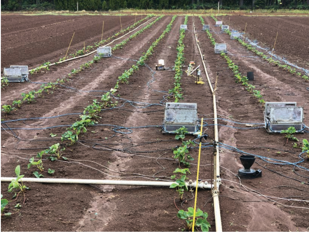
Figure 1. Field trial at Toolangi, Victoria evaluating the ability of different forms of chicken manure for offsetting fertiliser inputs in the production of strawberry runners. Automated chambers at the site continuously measure the release of gaseous forms of nitrogen and carbon from soils. Data from the trial will help support and validate the development of an app that will allow growers to better calculate the release of nutrients from organic amendments such as chicken manure. Photo credit: Scott Mattner
