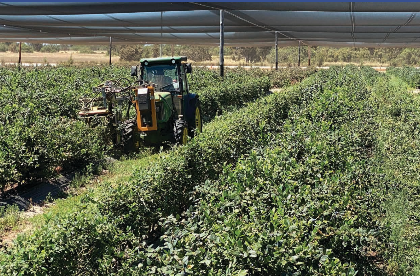
Figure 3. A sickle-bar hedger is used to prune plants annually after harvest to promote a targeted cropping window.
