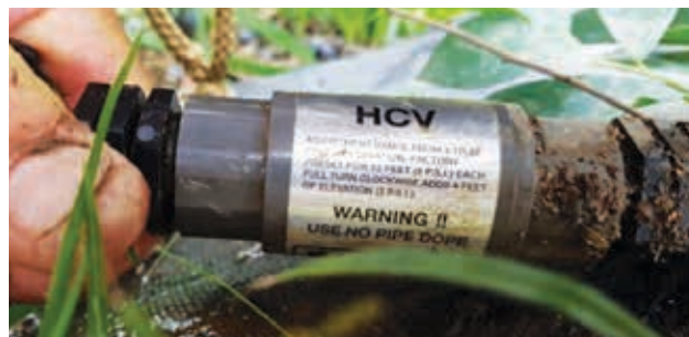
Figure 2. Check valves can reduce the drainage from mains to the lowest drippers. Photo credit: Rob Hoogers
