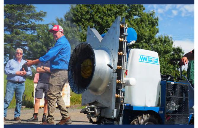
The self-propelled MM® tunnel sprayer unit that may suit small berry operations.
