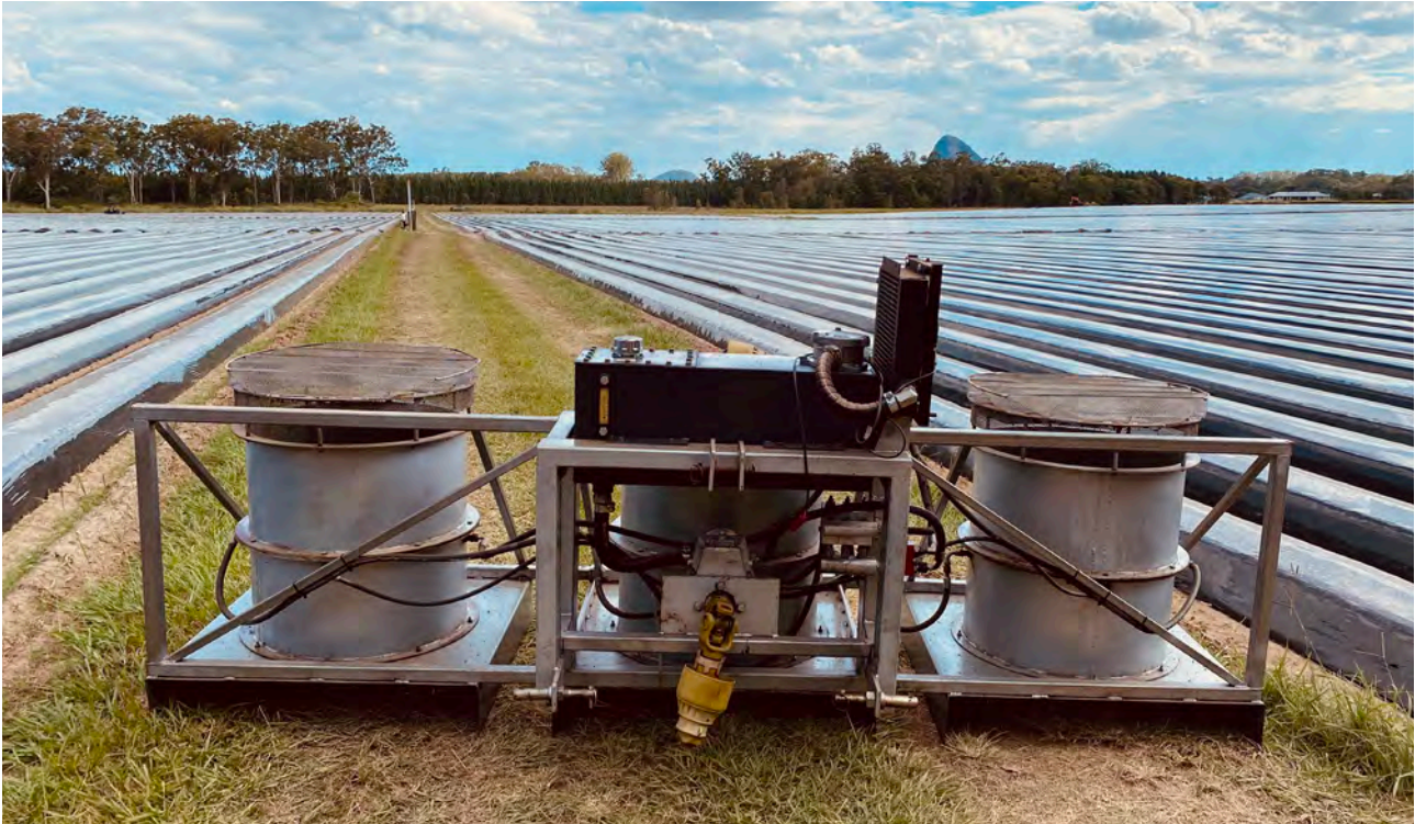
The bug vacuum unit can cover three rows in a single pass.
